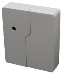
The RF1100 Glassbreak Transmitter is a wireless transmitter that detects breaking glass. It is equipped with two tamper switches and four glassbreak sensitivity settings. When there is no alarm activity, the RF1100 transmits a signal every 15 min, providing system supervision and battery status information. The RF1100 is compatible with the RF3212, RF3222, and RF3224 Receivers.
